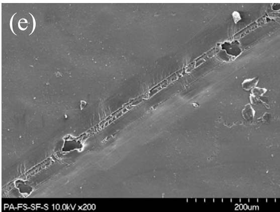
Figure S2. SEM images of active (a, c and e) and support (b, d and f) layer surfaces (PA-TFC membrane): before pressurization (a and b), after pressurization using tricot spacer (TS) (c and d) and feed spacer (FS) (e and f).
