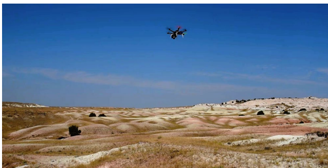
FIGURE 1 Unmanned aerial vehicle (UAV) starting autonomous mission over fossil-rich badlands in Wyoming, USA. Flight path is verified during the day and flown in detection mode at night. The UAV maintains height over the rolling hills using LIDAR
