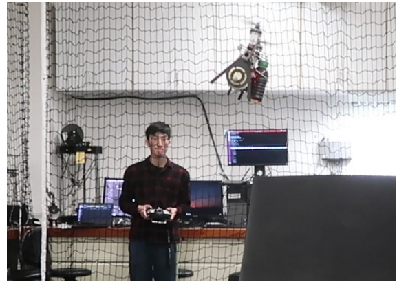
Fig. 17. The UAV carries a 324g water bottle on one side leading to a constant disturbance torque and model mismatch.
