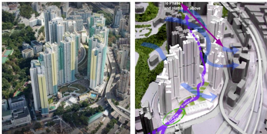
Figure 4 The Awarding-Winning Upper Ngau Tau Kok Estate Phase II & III purposefully designed to facilitate breeze and thermal comfort in open spaces. (left) An aerial photograph of the housing estate; (right) A design-stage physical model showing the site layout and breezeway 31
