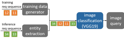
Fig. 1: An image classification service with an online learned VGG19 model. Grey models are stateless, and the blue model (i.e., the online learned VGG19) is stateful.
