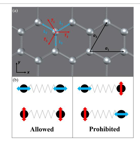
**Figure 1.** (a) A part of the mechanical graphene made by soft springs and rigid particles. (b) A schematic sketch of the allowed and prohibited vibrating mode transfer.
