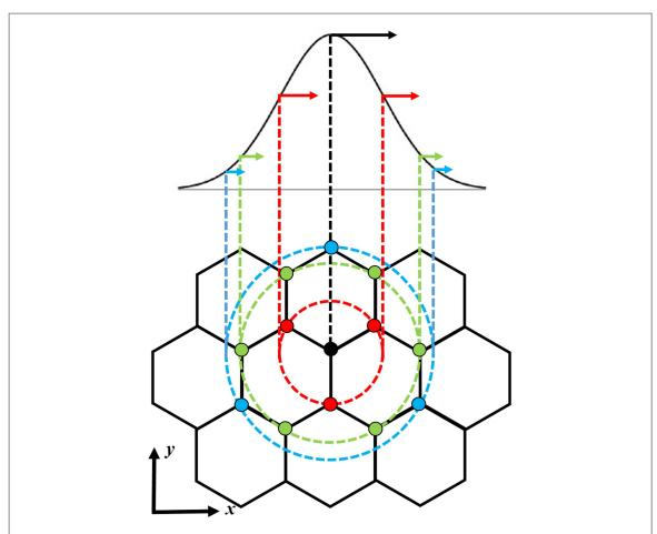
**Figure 3.** A schematic sketch of the initial displacement distribution. A Gaussian pulse  $A_0 \exp{[-(\mathbf{r} - \mathbf{R}_0)^2/\sigma^2]} \exp{[-t^2/\tau^2]} \exp{[i(\mathbf{k} \cdot \mathbf{r} - \omega t)]}$  is applied to the middle of the system, where it has a spatial deviation  $\sigma = 6a$  and time deviation  $\tau = 25$  ms. All the displacements are along x direction and the length of arrows denotes the corresponding displacements in the Gaussian pulse.
