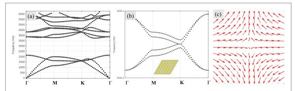
**Figure 5.** (a) The phononic band structure for tungsten carbide rods embedded in an aluminum background with lattice constant = 1 m. (b) Cavity-phononic crystal shows the dispersion being similar to figure 2(a). The inset demonstrates the geometry of a unit cell. (c) Spin texture of Dresselhaus SOC around K point. The orientation discrepancy from figure 2(d) is caused by the choice of primitive translation vectors.
