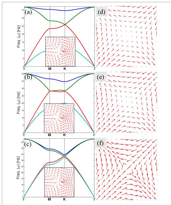
**Figure 2.** (a)–(c) The phonon dispersion for  $C_T = C_L/8$ ,  $C_L/3$ , and  $7C_L/8$  (M=10 g and  $C_L=4$  N m $^{-1}$ ). The insets are projected spin texture around  $\Gamma$  point. (d)–(f) are projected spin textures of third band for corresponding transverse elastic constants in the vicinity of K point. The length of arrows in spin textures indicates the strength of effective magnetic fields.
