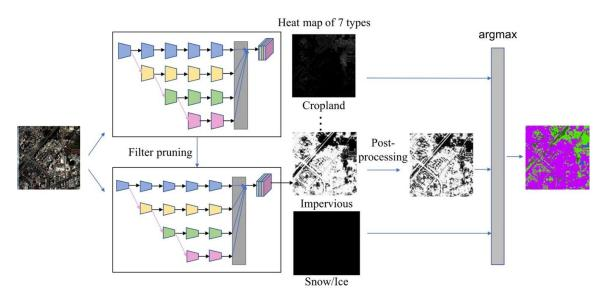
Figure 3. The overall workflow of our proposed method for land cover mapping.
