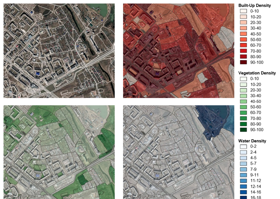
Figure 2. Evaluation of urban environmental indicators based on earth observation (EO) regarding built-up (upper right image), vegetation (lower left image), and water density (lower right image), using the SEN4RUS [39] approach. Here, an example of application in the city of Omsk, Russia is shown. Maps were created with QGIS software, version 3.4.4 ( www.qgis.org , accessed on 21 November 2019). Maps data: Google, Maxar Technologies.
