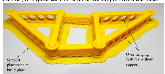
Figure 6. Non-assembly with normal support placed only at build plate
