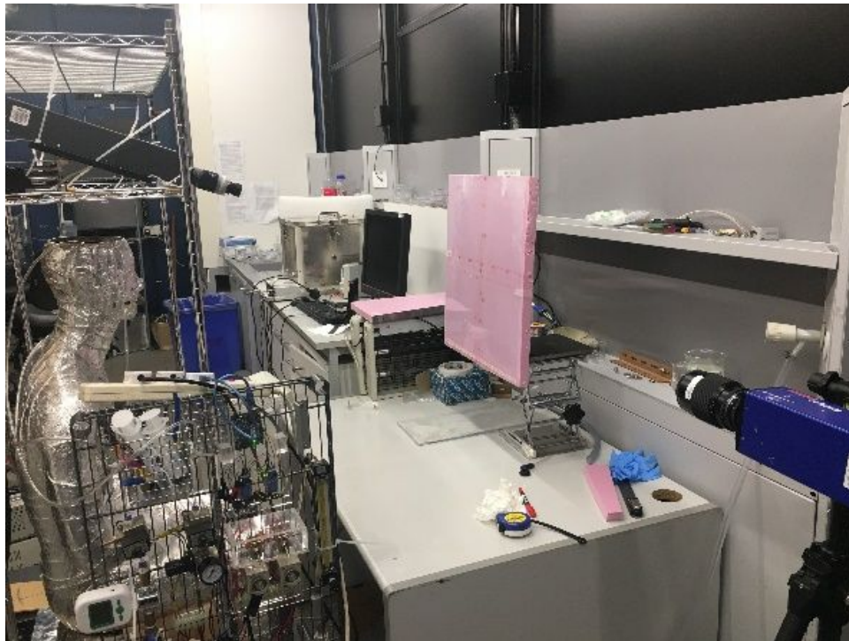
Figure 2S. PIV setup of the flow field measurement near the solid surface
