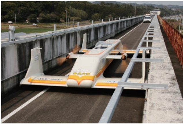
Fig. 4. Photograph of ART003R running on guideway.
