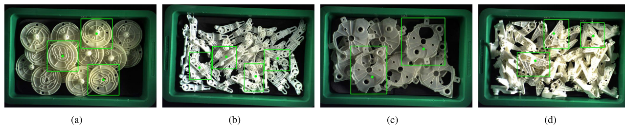
FIGURE 7. Training data. These data are made by labeling the bounding box and 2D feature point (green dots) of objects that are not occluded.
