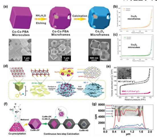
**Figure 10.** Pore structure design for MOF-derived materials.
