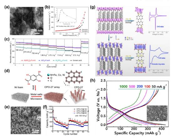
Figure 17. Tailoring pore structures of MOFs for metal-ion batteries.
