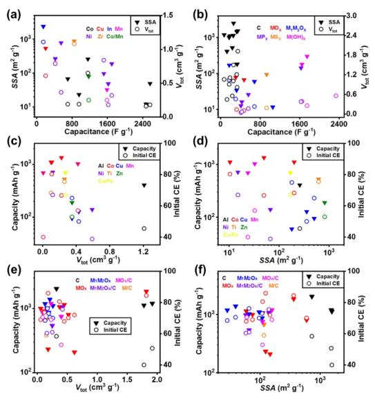
**Figure 21.** The correlations of structure/composition of (a,c,d) MOFs and (b,e,f) their derivatives to their performance for (a-b) supercapacitor electrodes and (c-f) LIB anodes. In figure a, c, and d, different colors denote MOFs bearing various metals. In figure b, e, and f, different colors denote MOF-derivatives of different kinds (C-carbon, M-metal, MO<sub>x</sub>-single-metallic oxides,  $M_1M_2O_x$ -bimetallic oxides).
