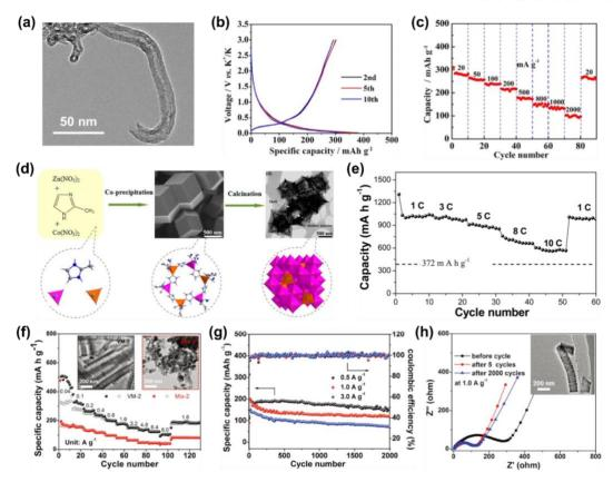
Figure 20. Tailoring pore structures of MOF-derived materials for metal-ion batteries.
