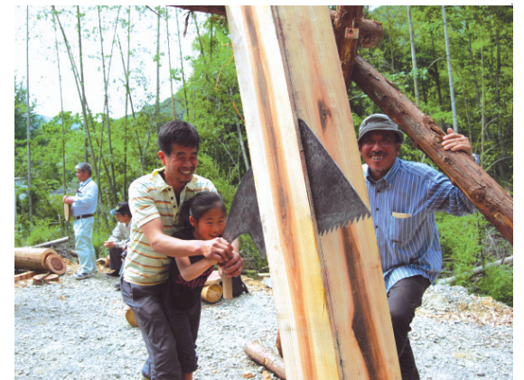
TESTING THE TRADITIONAL OGA (BIG SAW) METHOD
