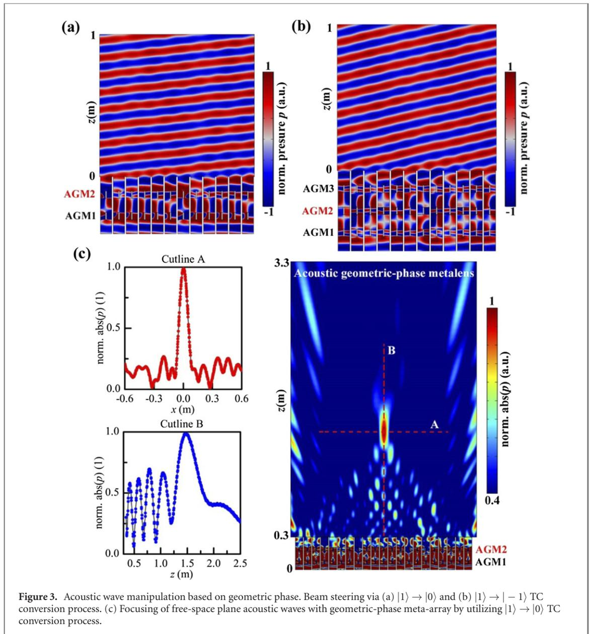
**Figure 3.** Acoustic wave manipulation based on geometric phase. Beam steering via (a)  $|1\rangle \rightarrow |0\rangle$  and (b)  $|1\rangle \rightarrow |-1\rangle$  TC conversion process. (c) Focusing of free-space plane acoustic waves with geometric-phase meta-array by utilizing  $|1\rangle \rightarrow |0\rangle$  TC conversion process.
