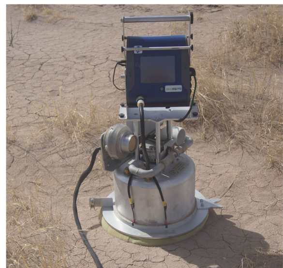
Fig. 3 PI-SWEL in test configuration on an undisturbed surface at the eastern beach area (EPL)
