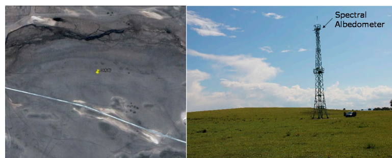
Figure 10. Field observation of the designed spectral albedometer. The left side shows the tower location from Google Earth on 30 April 2013. The site is homogeneous grassland, except for a road passing through the area. The right figure is the 20-m tower. The designed spectral albedometers are mounted atop the tower.
