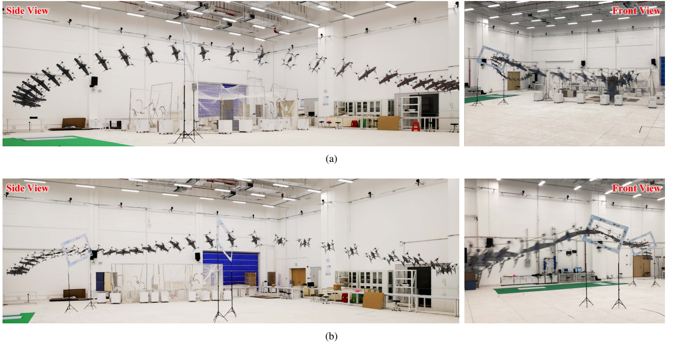
Fig. 10. Snapshot sequences of agile tail-sitter flight through narrow windows. (a) Flying through a single window in 10 m/s. (b) Flying through two consecutive windows in 8 m/s.
