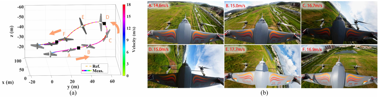
Fig. 23. Wingover: (a) illustration of the trajectory that is divided in two segments by three boundary points (black squares). Each segment is optimized by (48), (b) images from the FPV camera. Labels A-F denote different flight phases of the vehicle.
