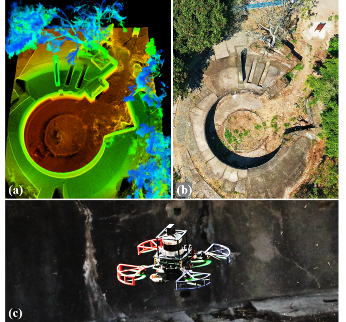
Fig. 1. Our proposed framework D-Map served as a real-time high-resolution occupancy mapping module for an autonomous UAV exploration task in an ancient fortress. (a) The high-fidelity point cloud collected by UAV. (b) A bird-view of the scene. (c) The aerial platform carried a 128-channel LiDAR (OS1-128) to conduct the exploration task. The accompanying video of this paper is available on Youtube: youtu.be/m5QQPbkYYnA .
