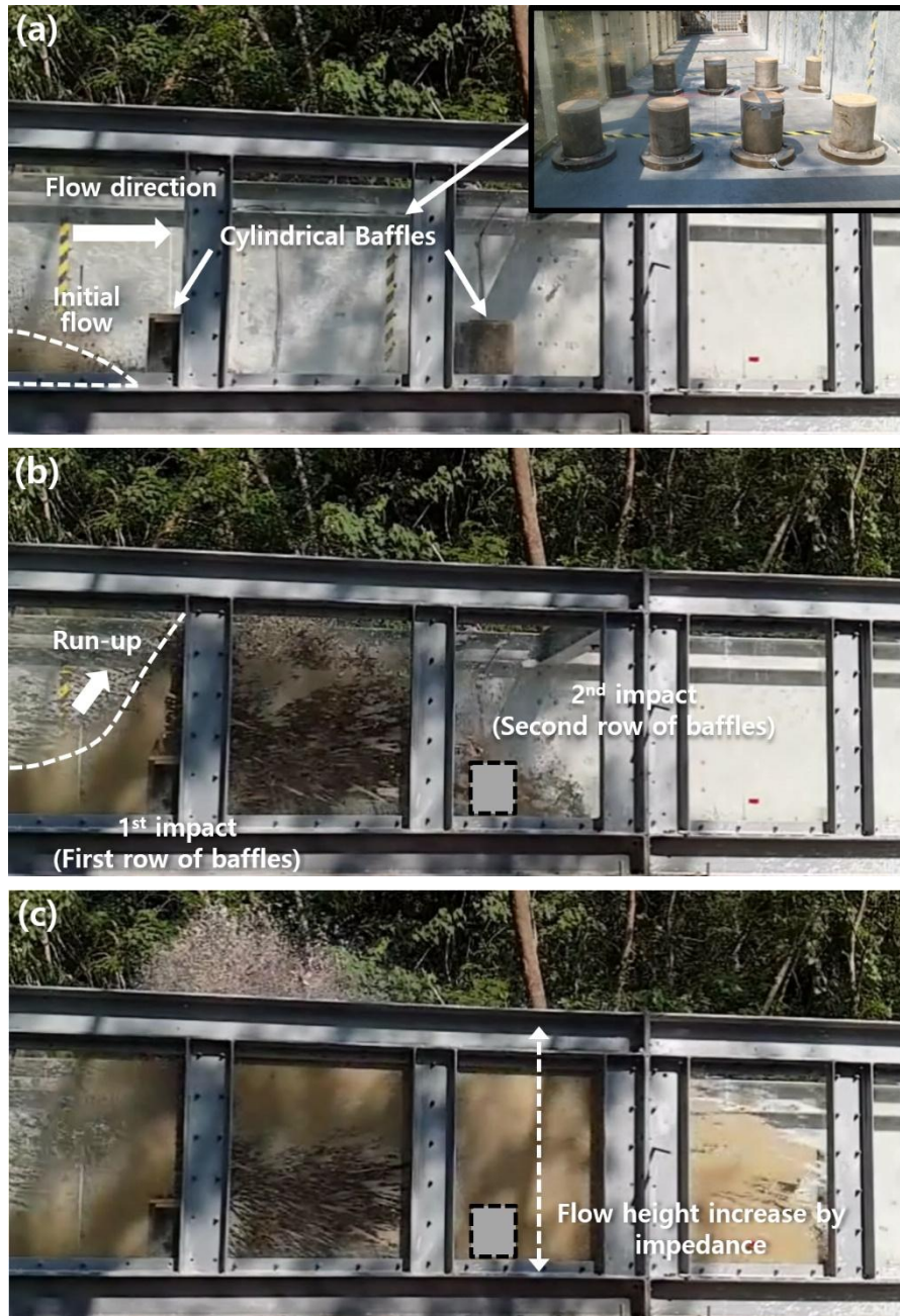
Fig. 19. Side-view flow kinematics of baffle array interaction in large-scale test (L_R2)
