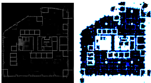
Figure 5: Line map and room map for repairing the floor plans predicted by the DNN.
