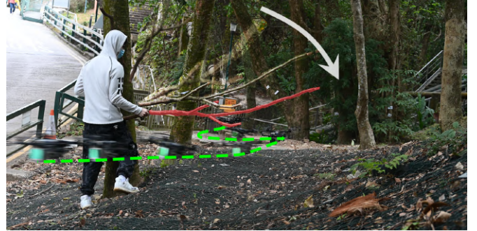
Fig. 1. Our system is able to detect and avoid dynamic small obstacles such as tree branches. The green dashed line is the path flied by the UAV, the white arrow indicates the movements of the tree branch. The current tree branch is highlighted in red. Video is available at https://youtu.be/mjtmpEYwQsI .
