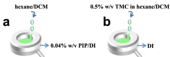
Fig. S5 1 min diffusion set up. (a) PIP diffuses from aqueous phase to organic phase.
