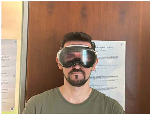
Figure 5. Virtual eyes projected onto the external screens of the Vision Pro (photo by Ruyu Yan).
