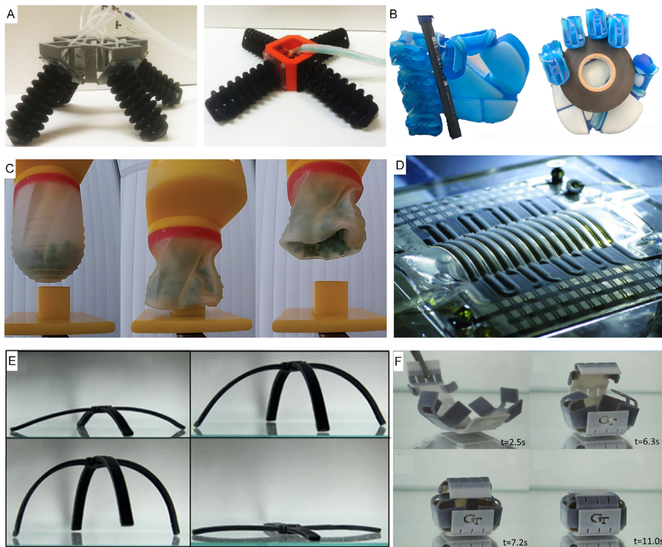
Figure 6. Smart structures printed by MJ. A) Quadruped robot with four pneumatic bellow legs. Reproduced with permission. [180] Copyright 2019, IEEE. B) MJ-printed soft robotic hand integrated 18 pneumatic pressure tactile sensors and 15 pneumatic bending actuators. Reproduced with permission. [184] Copyright 2022, IEEE. C) One-shot PolyJet-printed universal gripper based on granular jamming. Reproduced with permission. [186] Copyright 2022, Mary Ann Liebert Inc. D) The slug drive-integrated 14 channels and 28 soft actuators that generate a traveling wave for object transportation. Reproduced under terms of the CC-BY license. [188] Copyright 2020, The Authors. Published by Wiley. E) Reversible self-assembling and disassembling trestle composed of multishape active composites, a rubber matrix integrated with digital SMP fiber layers with different T_g . Reproduced under terms of the CC-BY license. [190] Copyright 2016, The Authors. Published by Springer Nature. F) 4D-printed sequential self-folding box with digital SMP hinges. Reproduced under terms of the CC-BY license. [192] Copyright 2015, The Authors. Published by Springer Nature.
