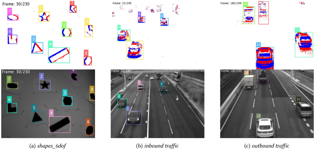
Fig. 11. Visualization of tracking results. The left-hand side of each figure shows the events accumulated from the 40 ms prior to the corresponding image frame and tracking results from REMOT. The right-hand side shows the corresponding image frame with the ground-truth bounding boxes.
