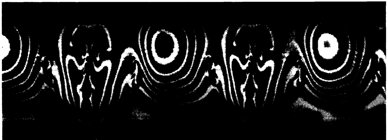
Fig. 14 Scanning moiré of the projected grating to depict contours of depth.
