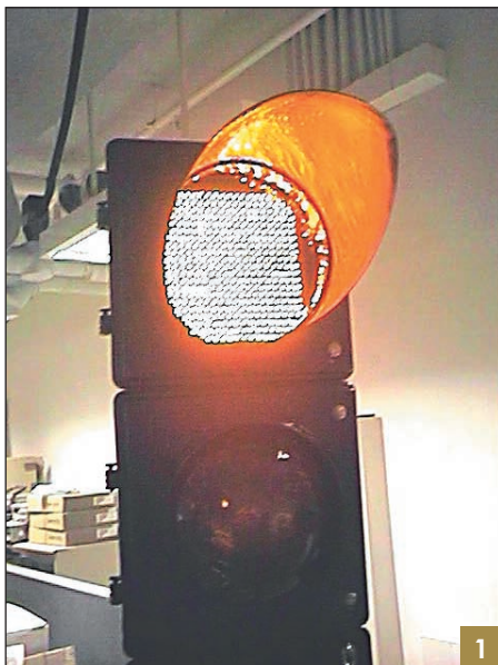
Photograph of a LED traffic light.
