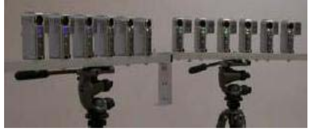
Figure 1. Two linear camera arrays, each consists of 6 JVC video cameras
