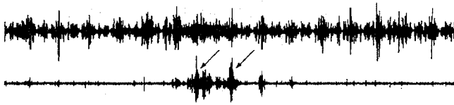
Fig. 2. The original (upper tracing) and wavelet-processed (lower tracing) DHS at 0.40 ml air infusion of Dog 2. The EHB are marked by arrows and confirmed by an experienced anaesthetist who listened to the playback signal of the recorded DHS.
