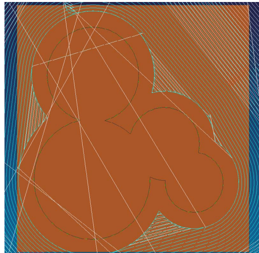
Figure 6. Smoother tool path generated by the proposed strategy
