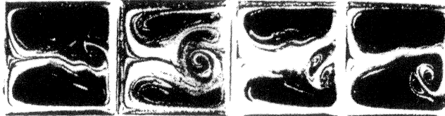
(a) Twisting Dean vortices at Re = 600 , Ro = 0 for Ts-A
