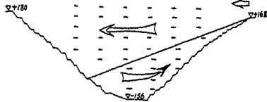
Fig. 2 A typical vertical airflow profile.
