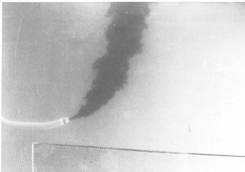
Fig. 1 a) Buoyant jet effluent issuing from a 1:11 hydraulic scale model of the Wah Fu sewage outfall. Jet velocity = 0.74 m/s, jet diameter = 0.1 m, relative density difference = 0.014. Densimetric Froude number = 6.3.
