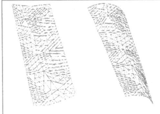
Figure 7 The surface triangular patch of the turbine blade (the left picture is the right ISO view and the right picture is the left ISO view)
