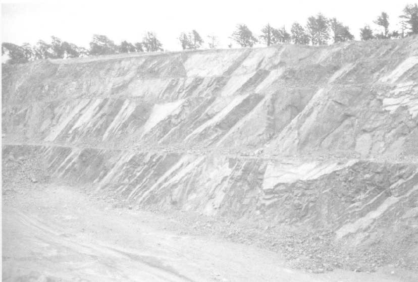
Fig. 8. Geological structural control by discontinuities on quarry faces
