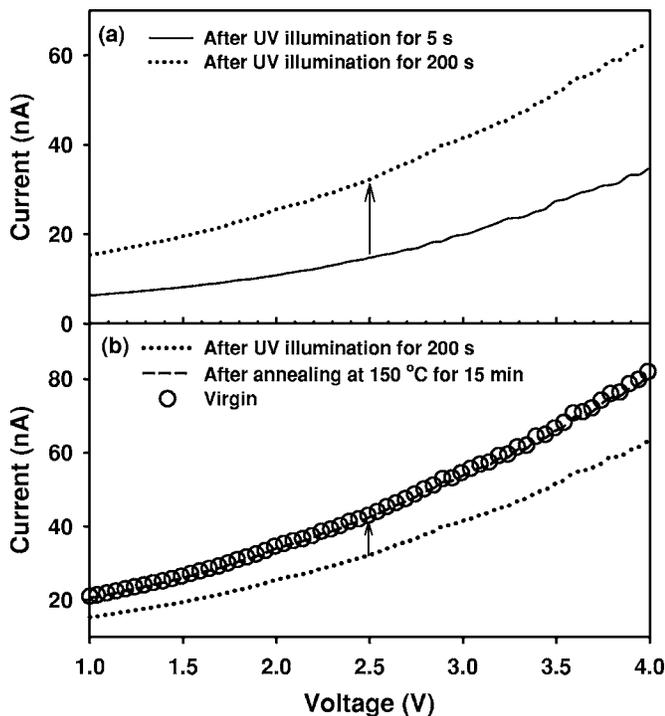
FIG. 5. (a) Partial recovery of the gate current after another UV illumination for 200 s from the situation of the UV illumination for 5 s. (b) Full recovery of the gate current after an annealing at 150 °C for 15 min in addition to the UV illumination for 200 s.
