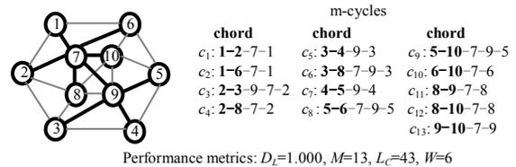
Fig. 1. HST for SmallNet (10 nodes, 22 links).
