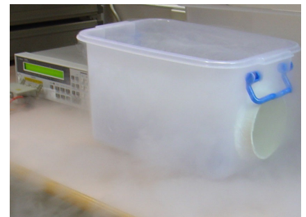
Fig 1. Resistance measurement of the HTS gradient coil in (a) room temperature and (b) liquid nitrogen
