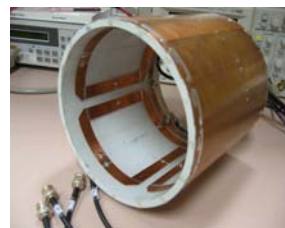
Fig.4. The photo of the four-channel microstrip loop array for 7T.
