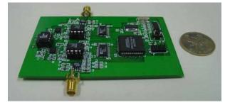
Fig. 2 MRI two channel FDM PCB prototype
